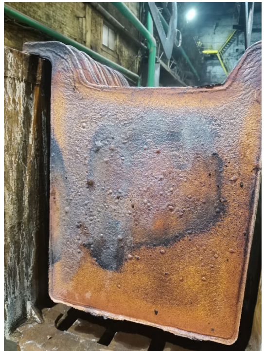
Figure 4 - Copper anode cast using "Lithoform" mould wash mark 900
