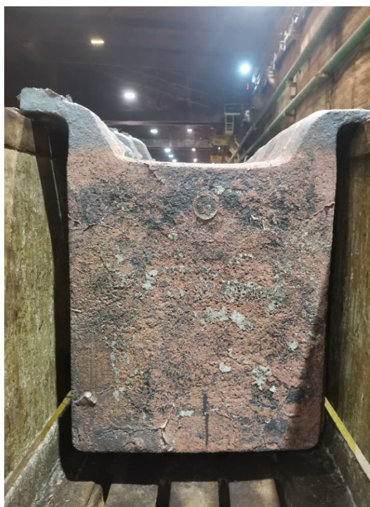
Figure 2 - Copper anode cast with chamotte mortar
