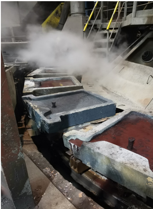
Figure 3 - Moulds treated with a suspension of mould wash "Lithoform" grade 900
