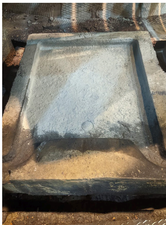
Figure 1 - The casting mould coated with chamotte mortar
